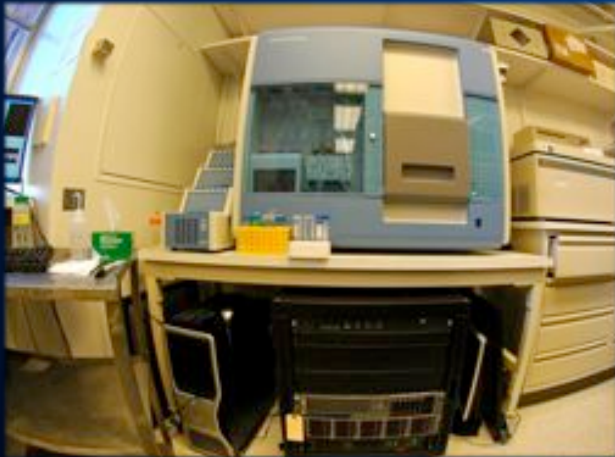
Self-contained lab-local cluster & storage for Illumina
