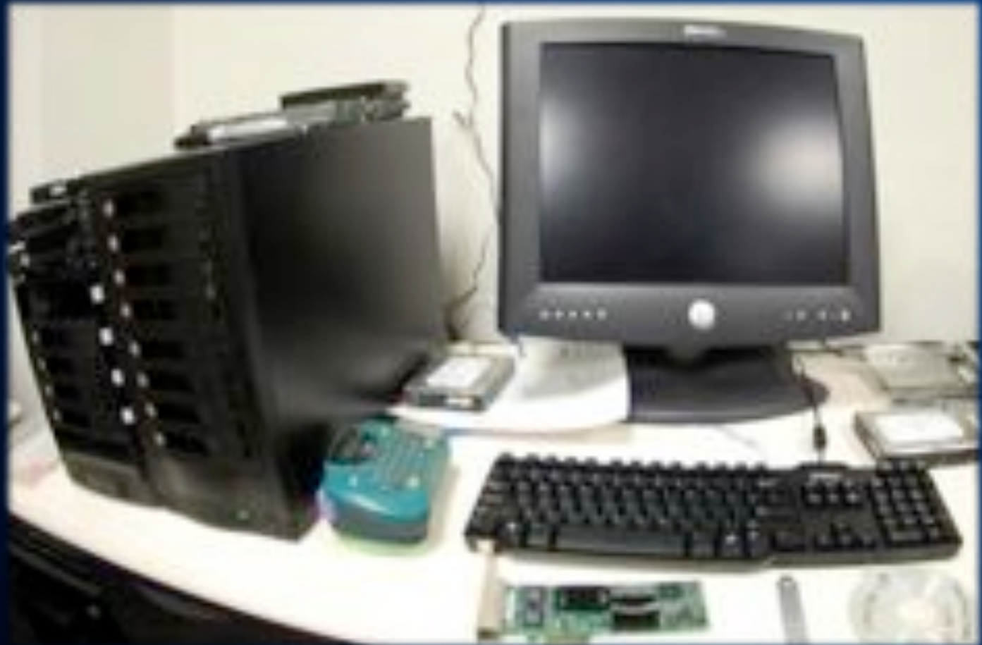
Data transfer station using hot-swap SATA disk bays
